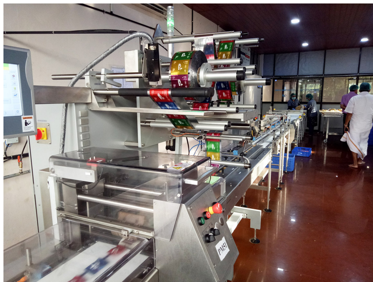
AUTOMATIC PEDDA PACKING MACHINE - WAYANAD DAIRY
