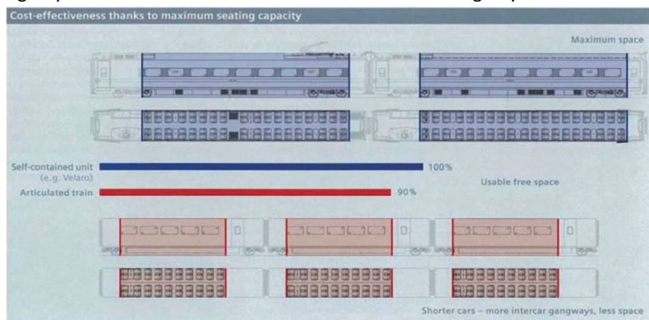
Figure 16: articulated and non-articulated trains
